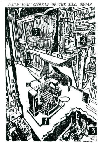
reg 2d individually. From the regulator the wind enters the wind-chest (T) ready to enter the pipes (U).
